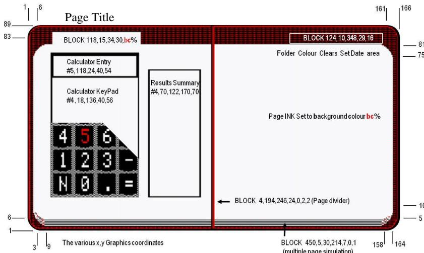
The additional WINDOW# channels are used for the Calculator Graphical representation.
