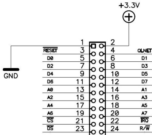
Position of Q68 Extension Bus on the Mainboard (green, Pin 1 marked):
