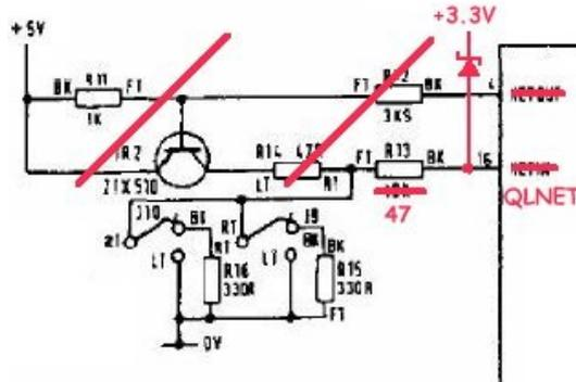
Note: If the Q68 is only used as network endpoint, only a 3.5 mm jack without switch, one 47 Ω, one 330 Ω resistor and a schottky diode (e.g. BAT43) are needed.
